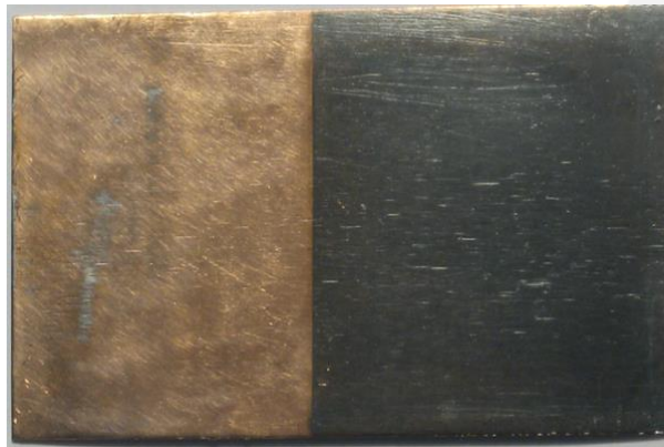
Figure 1: Copper coated with 200 nm of GCT - paint
