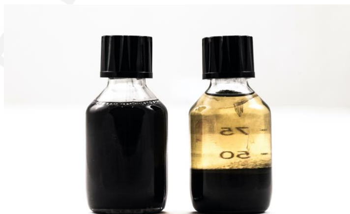
Figure 1: Example of graphene lubricant and graphene as additives in lubricant oil
