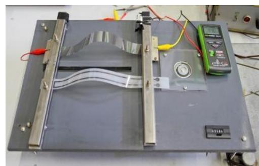
Figure 2: Fatigue test on graphene coated PET, sheet resistance measure before (left) and after (right) more than 50.000 cycles.
