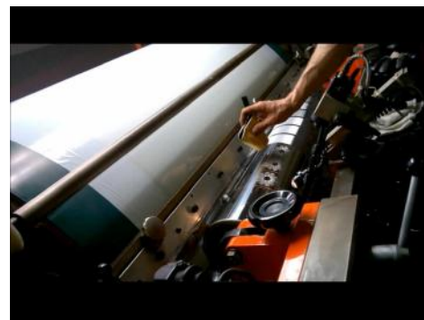
Inkjet and rotogravure printing of GNext XTInk on PET.
